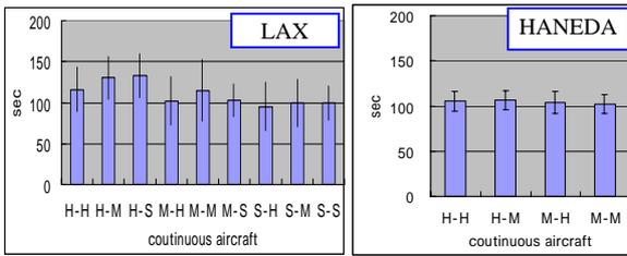
**Fig.4** Separation time at runway threshold ( Los Angeles International Airport and Haneda )
