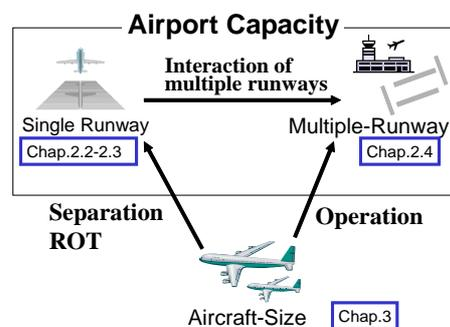
Fig.1 Relation of runway capacity and aircraft size
