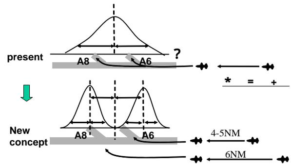
**Fig.3** Concept of new terminal air traffic flow control
