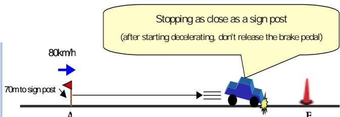
**Fig. 3-2** Decelerating experiment
