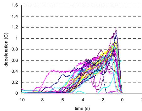
Fig. 3-7 Deceleration in simulator (Motion-ON)
